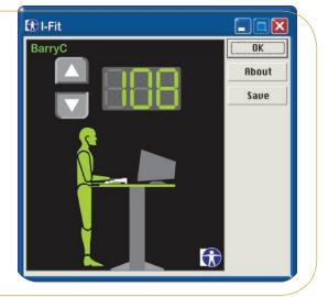
I-Fit's easy to use one-touch system provides a visual aid to ensure users find their correct setting which is indicated in "green". Desktop-mounted controls make it a snap to adjust the two worksurface heights to the correct numbers for each individual using the station.
